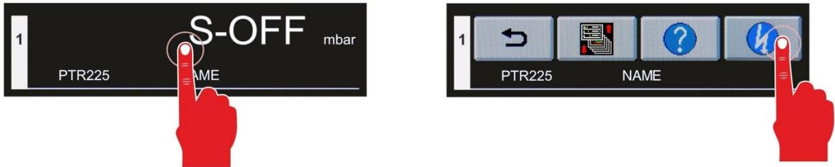
Figure 25 – Switching the high vacuum measurement circuit on
