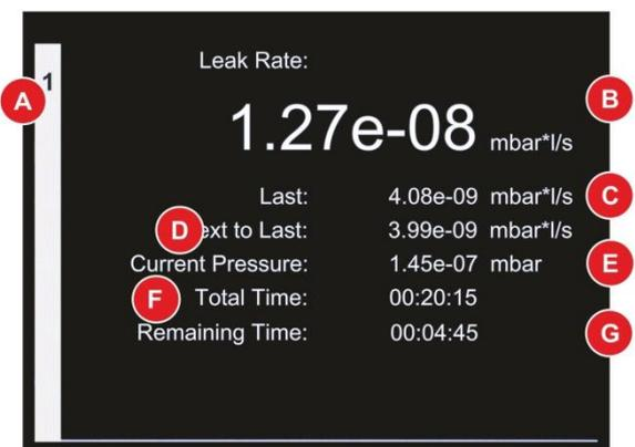
Figure 19 – Display mode Leak Test
