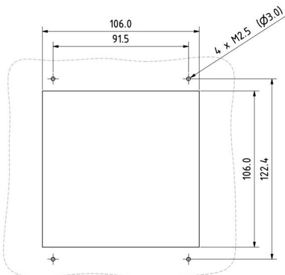
Figure 4 – Front panel cut-out (in mm)
