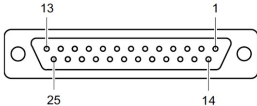
Figure 10 – Connection socket for relay output (SUB-D, 25-way)
