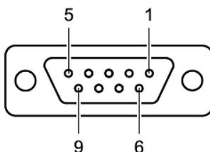
Figure 12 – Connection socket for interface (SUB-D, 9-way)
