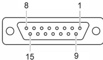
Figure 9 – Sensor connection (SUB-D socket, 15-way)
