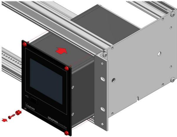
Figure 3 – Rack installation
