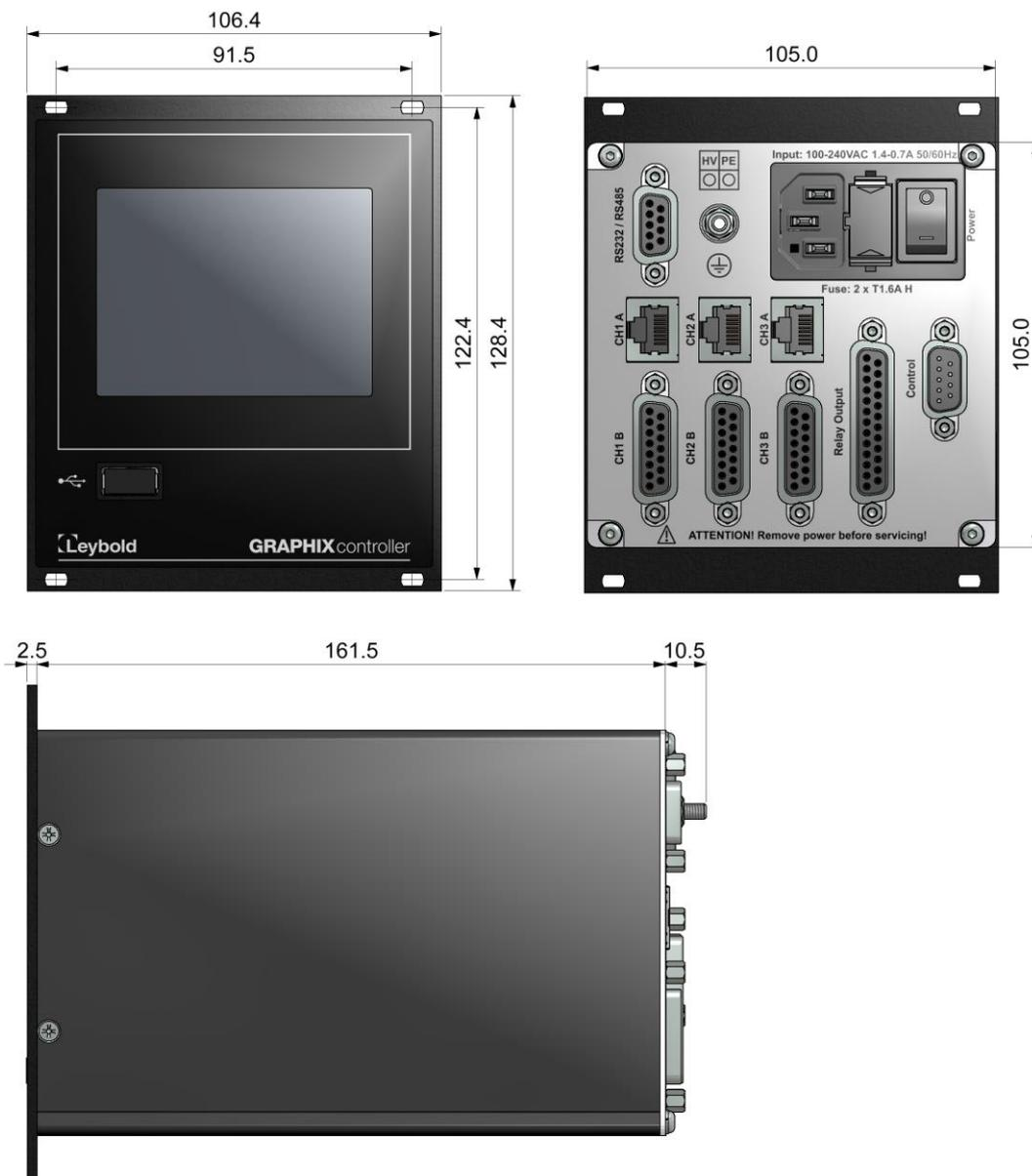
Figure 2 – Dimensions of the GRAPHIX controller (in mm)
