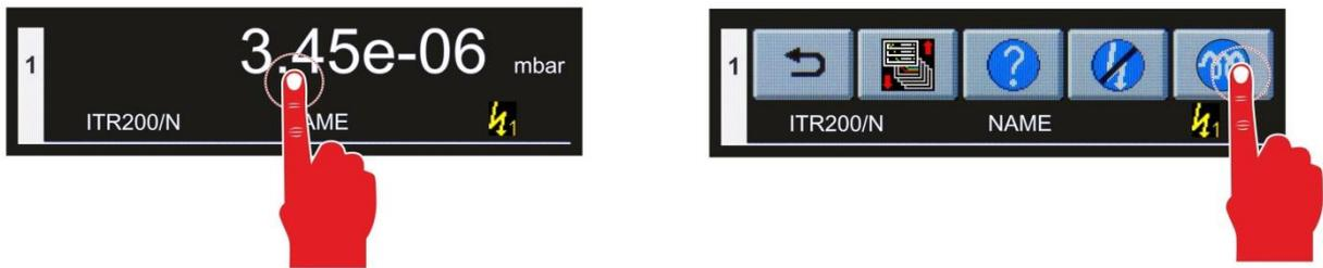
Figure 29 – Switching the degas function On
