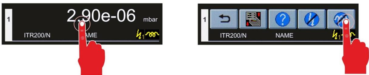
Figure 30 – Switching the degas function Off
