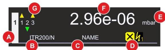
Figure 15 – Display field for a measurement channel
