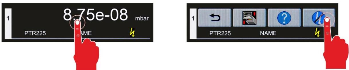
Figure 26 – Switching the high vacuum measurement circuit off
