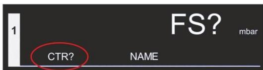
Figure 62 – Display of sensor type CTR?
