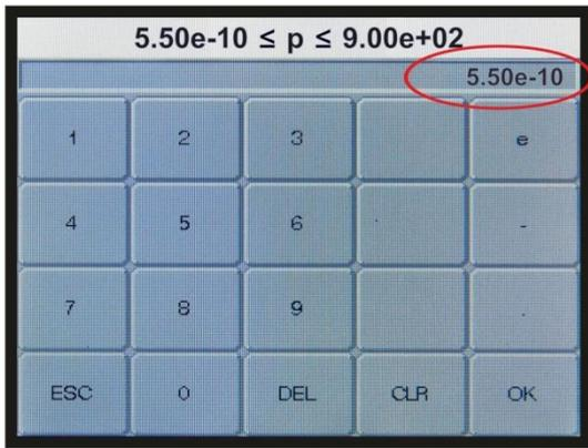
Figure 78 – Selection of the switching threshold value
